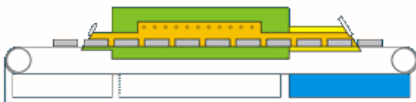
Mesh-Belt Furnace Scheme
